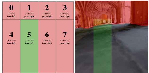
Figure 3. A demonstration of the robot's perception overlaid with both the traversability mask (in red) and the most-traversable octant (in green). In this case, the robot predicts to turn left using the Bottom-Heavy Octant heuristic.
