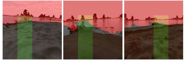
Figure 5. Three traversability segmentations and heuristic selections with water in the vicinity. The two on the right exhibit the peninsula effect.
