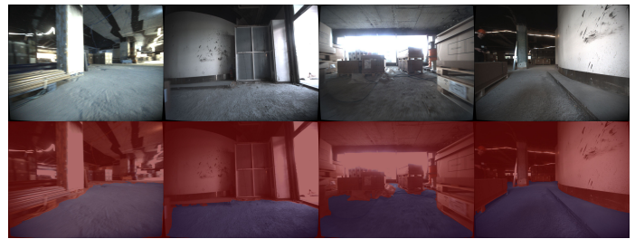
Fig. 5. Randomly selected traversability masks generated using the prompts “something an Anymal robot could walk on” and “other”. Images were taken on a typical large construction site by an Anymal D, and the masks were generated using the largest OVSeg model. The rightmost mask shows a step being classified as traversable
