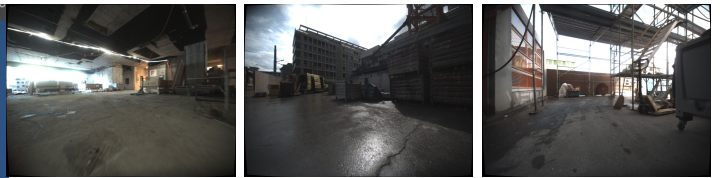
Fig. 9. Example of data taken from the RGB front wide angle camera, taken from the first mission. These images were taken in conditions identical to use-case, i.e., the robot is in active motion (no time to look pretty); the images arrive in the resolution 1080x1440 as compressed jpg images—we are not sure what the compression ratio is.
