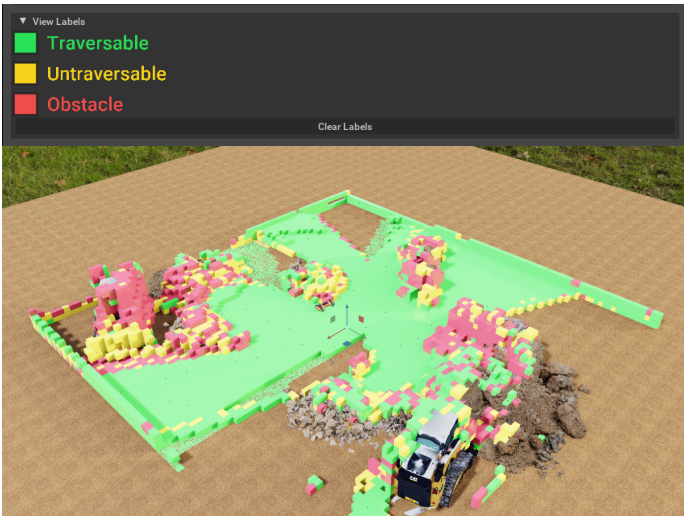
Fig. 4. Visualizing the Voxel Segments. The colors correspond to the classes as defined in the extension. Classification was performed online using the RGB and depth images taken by the ANYmal after walking it around in simulation.
